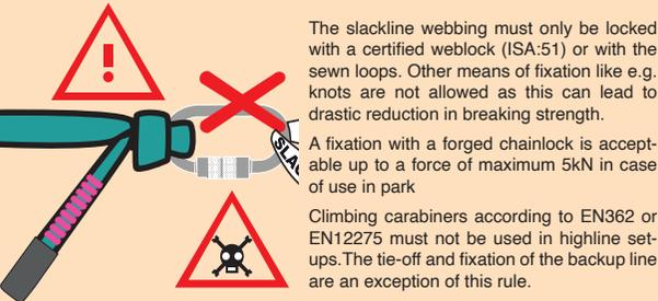
The slackline webbing must only be locked with a certified weblock (ISA:51) or with the sewn loops. Other means of fixation like e.g. knots are not allowed as this can lead to drastic reduction in breaking strength.
