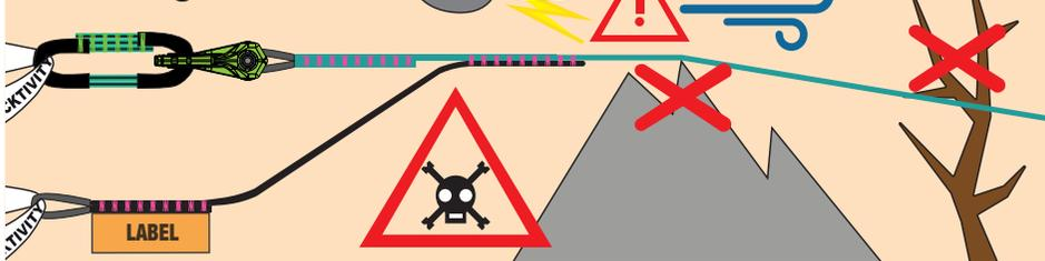
The slackline webbing must be installed hanging freely. No support. Make sure to leave enough space to branches and other obstacles so that no contact is possible even when the line is being moved heavily to different sides.
