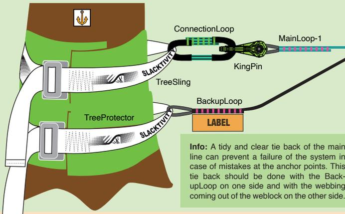
**Info:** A tidy and clear tie back of the main line can prevent a failure of the system in case of mistakes at the anchor points. This tie back should be done with the BackupLoop on one side and with the webbing coming out of the weblock on the other side.
