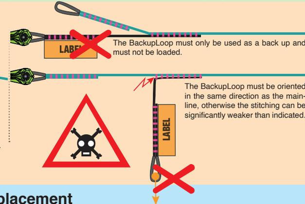
The BackupLoop must only be used as a back up and must not be loaded.
