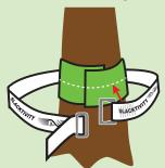
1. Fix the TreeSling to the tree protector with help of the Velcro and put it around the tree. Always use with a TreeProtectionto protect the trees but also to protect the TreeSling from sharp edges and abrasion.
