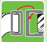
2. If needed, adjust the position of the locking plates so that both plates can be clipped into one another. Push the smaller metal plate in a tilted position through the bigger one to clip the metal plates into one another. The SLACKTIVITY print must be on the outer side of the sling and therefore visible. The sling must not be twisted. The metal plates must be placed on the back side of the tree - in the opposite direction of the slackline.
