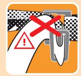
The webbing-tail coming out of the locking plates must not be threaded through the big metal plate as the TreeSling might open up to the stopper otherwise.
