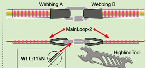
Two webbings (A+B) can be connected with a 8-10mm oval quicklink connecting the two end loops (MainLoop-2). The quicklink must be screwed tight with the HighlineTool (or a similar tool) in a way that it cannot be opened by hand anymore. For optimal performance we recommend the 8mm INOX quicklink of Maillon Rapide.
